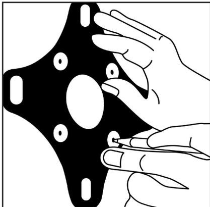
Use a drill to make holes for the anchors.
